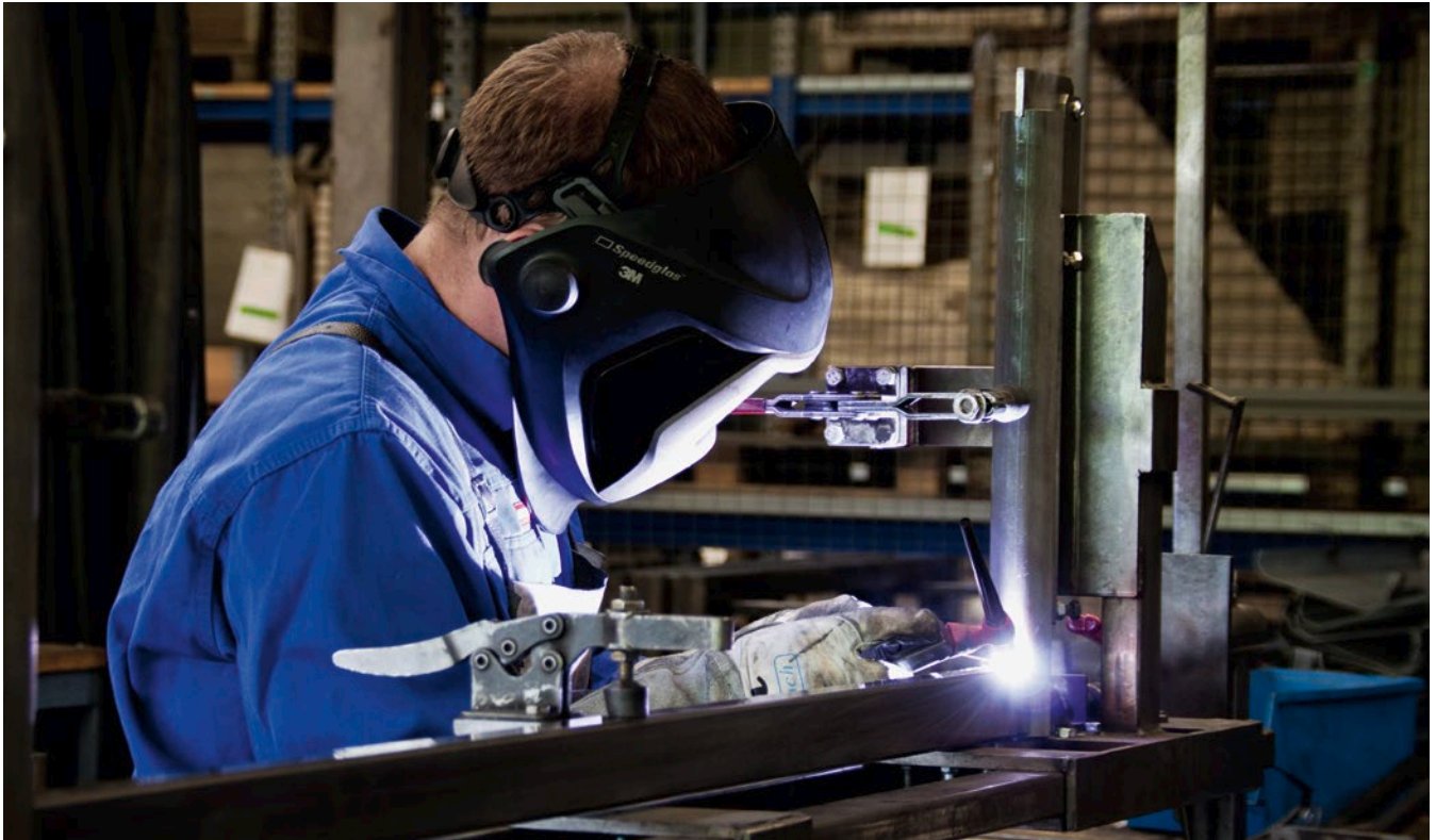
The steelworking department produces precise and durable frames from tubes and sheets for Wilkhahn tables. Special equipment ensures safety while welding; maintenance and inspection of the machinery protects the environment.
